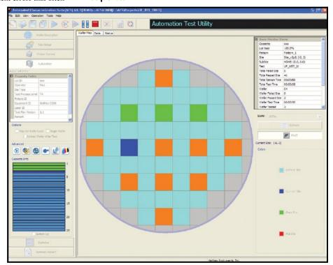
ACS software provides wafer- and cassette-level automation capabilities compatible with semi and fully automatic probe stations.
