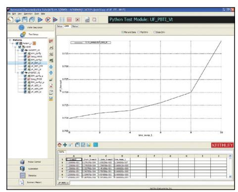
The Model 4225-PMU/4225-RPM's combination of superior speed and sensitivity allow characterizing voltage threshold ( $V_{\tau}$ ) directly with high-speed  $I_{D}$ - $V_{G}$  sweeps. Measuring  $V_{\tau}$  directly makes it unnecessary to correlate the single-point  $I_{D}$  measurement to actual  $V_{\tau}$  levels.
