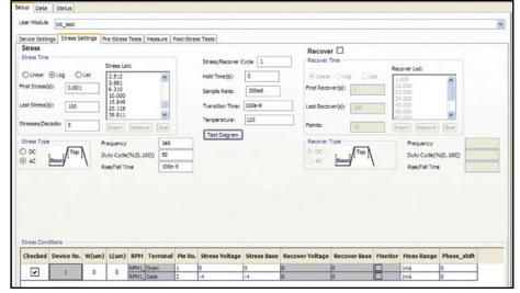
Define stress timing and stress conditions easily using familiar parameters like timing – log, linear, custom list; measurements per decade; AC or DC stress; optional recovery test sequence; and test sample rate (speed).
