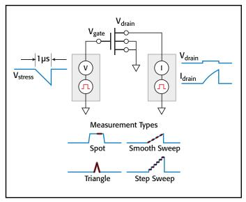
The Ultra-Fast BTI test software module supports spot, step sweep, smooth sweep, and sample measurement types. Each type's timing is defined by the test sample rate and the individual measurement settings. The software module also provides control over the voltage conditions between each element in the test sequence, for maximum flexibility and ease of use, even when defining complex test sequences.
